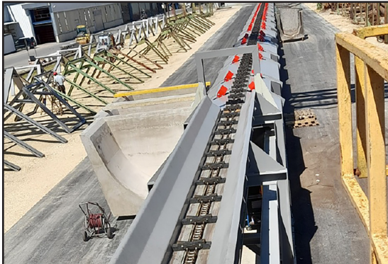
Tree trunk transport chain in a sawmill.
